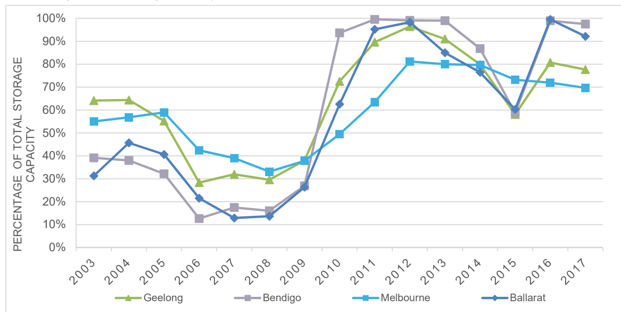
Figure 2-10 Water in reservoirs for major urban centres at the end of October, each year from 2003 to 2017, as a percentage of total storage capacity
